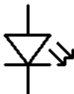
Figure 1 – Schematic Symbol for an LED
