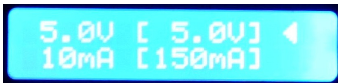
Default mode with variable Voltage and Current (Current limit is 150mA, actual is 10mA)
